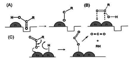
Fig. 5 Hydrogenation of carboxylic acid ensuing through (A) the interaction of the oxygen atom of the carbonyl group with the oxygen vacancies created by hydrogen spill-over by Pt metal, (B) the interaction of the oxygen atom of the carbonyl group with Re on the surface of the PtRe/ $TiO_2$  bimetallic catalyst, and (C) the decarboxylation of carboxylic acid on the surface of Re on the surface of the PtRe/ $TiO_2$  bimetallic catalyst (adapted from ref. 40).
