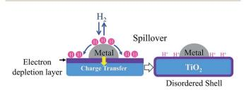
Fig. 2 An example of hydrogen spill-over involved in hydrogenation of metal  $TiO_2$ .
