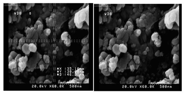
Fig. 2 SEM image of Cu(II) immobilized on Fe<sub>3</sub>O<sub>4</sub>@SiO<sub>2</sub>@L-arginine
