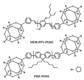
Chemical structures of MEH-PPV-POSS and PHF-POSS
