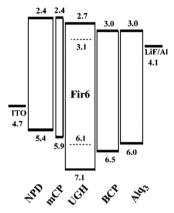
Fig. 3 The energy level diagram (units: eV) for the device: ITO/NPD (400 Å)/mCP (100 Å)/Fir6:UGH (10%, 250 Å)/BCP (150 Å)/Alg<sub>3</sub> (250 Å)/ LiF/Al. Reproduced with permission from ref. 47, Copyright 2004 American Chemical Society
