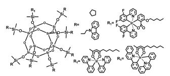
Fig. 18 Chemical structures of iridium-complex anchored polyhedral oligomeric silsesquioxane (POSS) macromolecules.
