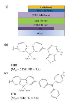
Fig. 3 (a) Schematic illustration showing the device architecture investigated and individual layer thicknesses, (b and c) molecular structures, molecular weight  $(M_w)$  and polydispersity (PD) information for F8BT and TFB.
