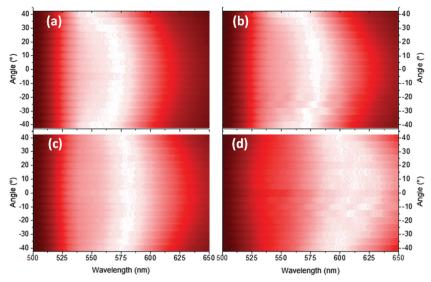
Fig. 5 Intensity maps highlighting the shift in EL wavelength measured with changing viewing angle  $(\pm 40^{\circ})$  for bilayer devices with a TFB thickness of (a) 40 nm, (b) 50 nm, (c) 60 nm and (d) 100 nm of TFB.
