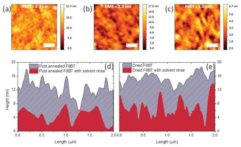
Fig. 2  $2 \times 2 \mu m$  AFM images of (a) slow cooled F8BT after annealing above  $T_m$ , (b) after cyclohexanone rinse (c) following TFB addition (d and e) roughness profiles of annealed and dried at 90 °C F8BT showing the reduction in roughness observed after solvent rinse.
