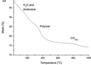
Fig. 3 (A) FTIR spectra of CaP capsules (red line), and CaP capsules annealed at 1000 °C (black line). (B) TGA curve of CaP capsules.
