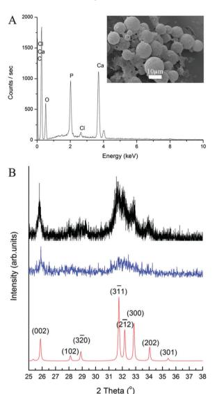
Fig. 4 (A) EDX spectrum and SEM micrograph of CaP capsules. (B) XRD patterns of CaP capsules as synthesized (blue line), CaP capsules annealed at  $600\,^{\circ}\text{C}$  (black line), and simulated powder pattern of single crystal hydroxyapatite (red line).
