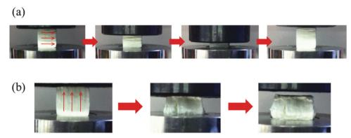
Fig. 9 Images showing the compression behaviour of the freeze cast 60 wt% organic hybrid scaffolds fabricated at a cooling rate of  $10 \, ^{\circ}$ C min $^{-1}$ ). Scaffolds compressed (a) perpendicular to the freezing direction, which demonstrate the highly elastic behaviour, and (b) compressed parallel to the freezing direction by a compressor, which shows the rupture formation and failure to recover after the compression. The arrows on the sample indicate the freezing direction.
