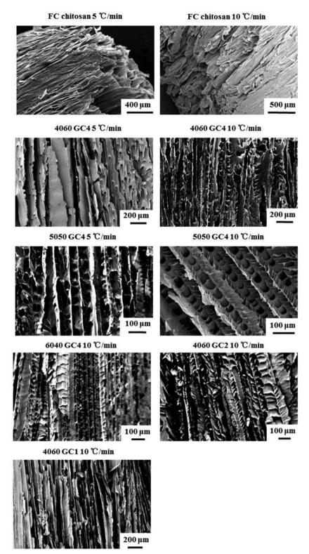
Fig. 7 SEM images of freeze cast scaffolds fabricated with various compositions and cooling rates. Cross-sections parallel to the freezing direction, which show the oriented pore structures.
