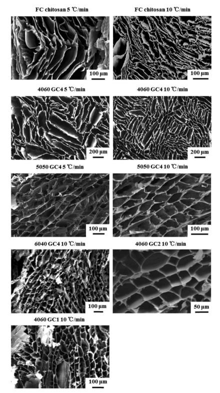
Fig. 6 SEM images of freeze cast scaffolds fabricated with various compositions and cooling rates. Cross-sections perpendicular to the freezing direction, which show the cellular pore structures.
