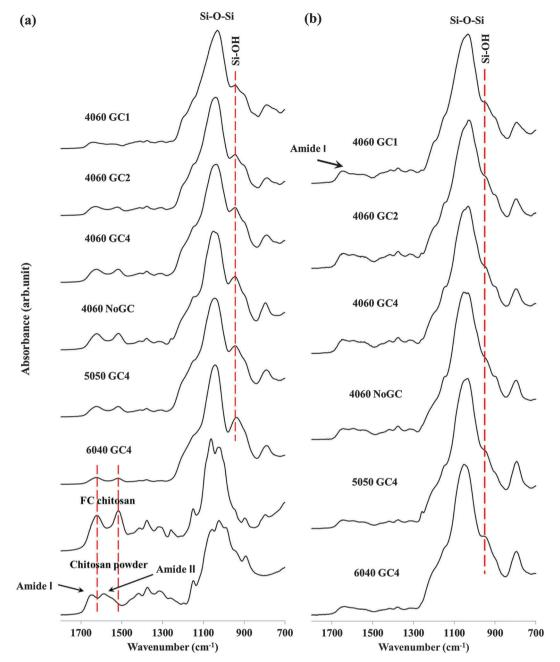
Fig. 4 FTIR spectra of (a) commercial chitosan powder and freeze cast scaffolds with various compositions and of (b) freeze cast scaffolds with various compositions after four-week immersion in TRIS buffer solution.
