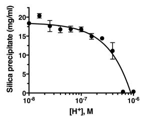
Fig. 3 Silica precipitation is linear with respect to proton concentration. Data are mean  $\pm$  s.d. from three independent experiments, shown on a log scale for clarity with a linear fit ( $R^2 = 0.9$ ). All reactions were 50 mM silicic acid, 2.5 mM R5
