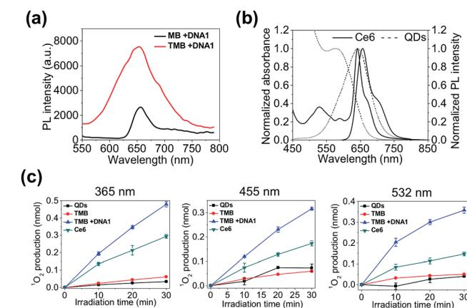
**Fig. 3** *In vitro* evaluation of theranostic efficacy of TMB. (a) Photoluminescence spectra of DNA1-activated TMB and MB (same Ce6 concentration) excited at 405 nm. (b) Normalized absorption spectra and photoluminescence spectra of CdTe/CdS/ZnS QDs and Ce6 molecules. (c) Quantification of  ${}^1\text{O}_2$  generation by QDs, TMB, DNA1-activated TMB, and free Ce6 (same Ce6 concentration) irradiated at 365 nm, 455 nm, and 532 nm for 10, 20, and 30 minutes.
