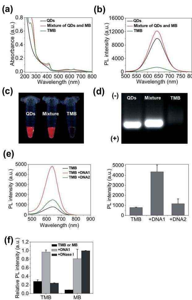
**Fig. 2** TMB construction and activation. (a) Absorption spectra; (b) photoluminescence spectra; (c) photographs under UV excitation; (d) agarose gel electrophoresis of CdTe/CdS/ZnS QDs, mixture of QDs and MB (without TCEP reduction), and TMB. (e) Activation of TMB with perfect-matched DNA1 and single-base-mismatched DNA2 measured by photoluminescence spectra. (f) Digestion of TMB and MB with DNase I measured by the PL intensities of the probes. DNA1-activated TMB and MB are used as controls.
