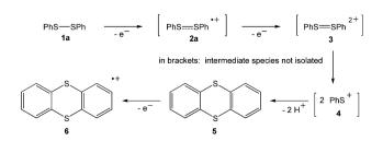
${\bf Scheme\ 1}\quad {\bf Oxidation\ of\ diphenyldisulfide\ in\ conc.\ sulfuric\ acid.}$
