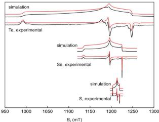
Fig. 3 Field-sweep EPR spectra for 17a (E = S) 17b (E = Se) and 17c (E = Te) measured in frozen CH<sub>2</sub>Cl<sub>2</sub>/THF solution (1:1), along with the corresponding simulations
