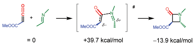
Scheme 8 DFT computed (DFT-D3, BP86, def2-TZVP) uncatalysed coupling of the free (uncoordinated) ketene and imine substrates.
