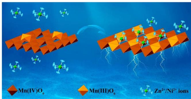
Figure 6 Electrodes made from birnessite, a manganese oxide mineral, captured  $Zn^{2+}$  and  $Ni^{2+}$  by reducing the manganese within the birnessite from Mn(IV) to Mn(III). This reduction is accompanied by the insertion of  $Zn^{2+}$  or  $Ni^{2+}$  into the birnessite. Reproduced from ref. 112 with permission from Elsevier, copyright 2019.
