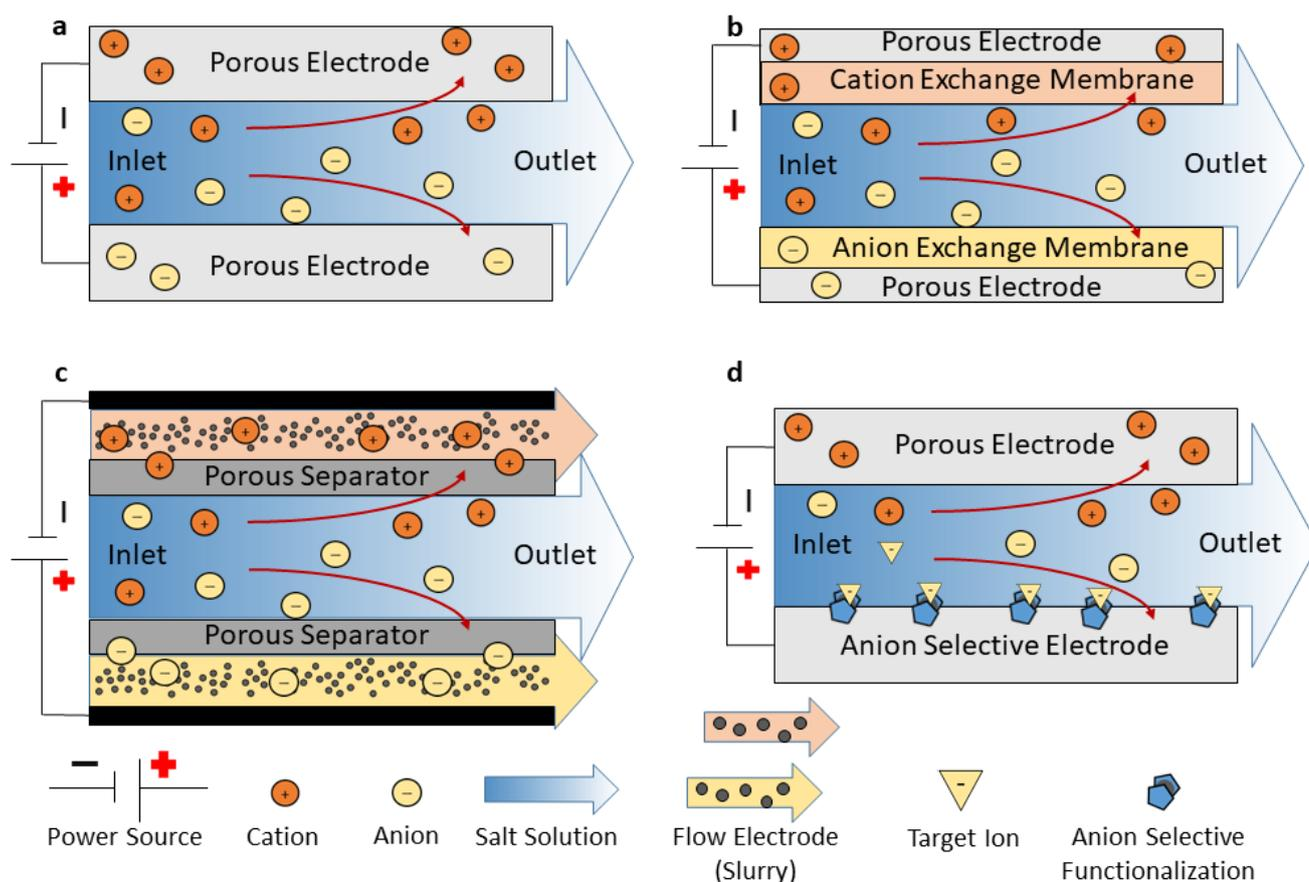
Figure 1 - Schematic of various CDI and electrosorption processes. Electrosorption processes are modular and can be combined with other ion separation techniques such as (b) membrane processes and can be (c) operated with flow electrodes. (d) Recent trends in electrosorption focus on designing materials that can selectively remove target ions.
