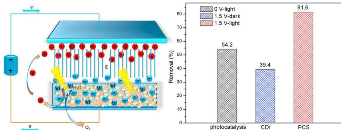
Figure 3 Synergistic conversion and removal of Cr by a photocatalysis and capacitive deionization system (PCS). Cr(VI) species are anionic and only attracted to the anode in a CDI system. By photocatalytically reducing Cr(VI) to Cr(III), which are typically cationic species, both the cathode and anode could be utilized to capture Cr. Reproduced from ref. 73 with permission from Elsevier, copyright 2019.
