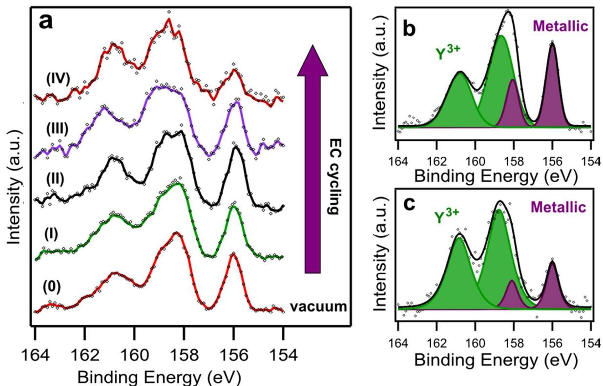
**Figure 2: Dealloying of  $Pt_xY$  nanoparticles.** (a) Y 3d XPS spectra of  $Pt_xY$  nanoparticles under vacuum (0) and under water vapor pressures of 5 Torr as a function of potential cycling (I-IV) (b) Curve fitted Y 3d XPS spectrum before potential cycling. (c) Curve fitted Y 3d XPS spectrum after potential cycling. The incident photon energy was 700 eV.
