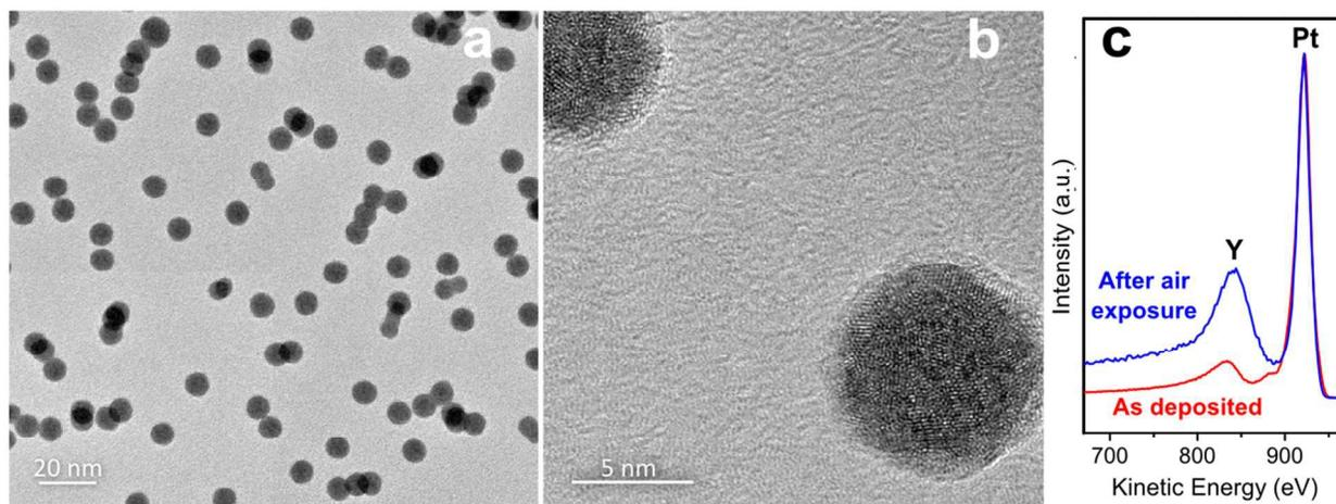
**Figure 1: As-deposited  $Pt_xY$  nanoparticles characterization.** Representative TEM images of size-selected 9 nm  $Pt_xY$  nanoparticles at a lower (a) and higher (b) magnification. (c) ISS spectra of 9 nm  $Pt_xY$  nanoparticles before and after exposure to air. The peaks at  $\sim 920$  eV and  $\sim 830$  eV correspond to Pt and Y respectively.
