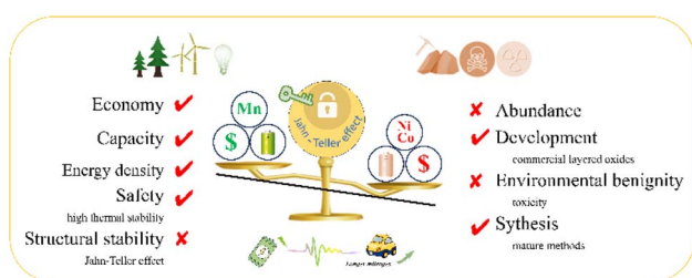
Fig. 8 Comparison of commercialized NCM cathode materials and representative Mn-based materials.
