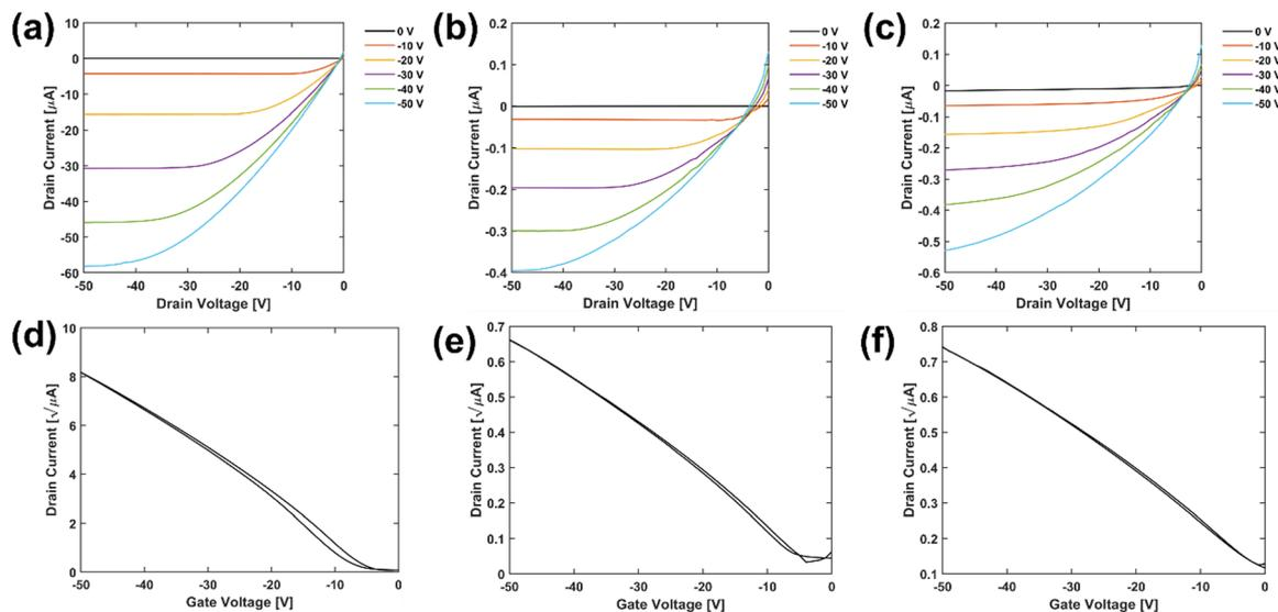
Fig. 3 The output characteristics of OFETs comprising (a) PDPPP4T on XLPS/SiO<sub>2</sub>, (b) P1BT1:1 on XLPS/SiO<sub>2</sub>, and (c) P3BT1:1 on XLPS/SiO<sub>2</sub>, and the square root transfer characteristics of OFETs comprising (d) PDPPP4T on XLPS/SiO<sub>2</sub>, (e) P1BT1:1 on XLPS/SiO<sub>2</sub>, and (f) P3BT1:1 on XLPS/SiO<sub>2</sub>.
