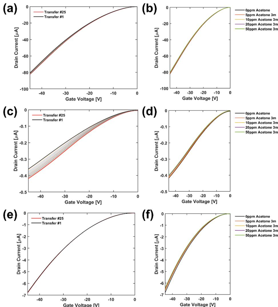
Fig. 4 PDP4T on XLPS/SiO<sub>2</sub> OFETs: (a) drift current in air and (b) response to acetone gas exposure. **P3BT1:2** on XLPS/SiO<sub>2</sub> OFETs: (c) drift current in air and (d) response to acetone gas exposure. P1BT: PDP4T blend (25 : 75 by weight) on XLPS/SiO<sub>2</sub> OFETs (e) drift current in air and (f) response to acetone gas exposure.
