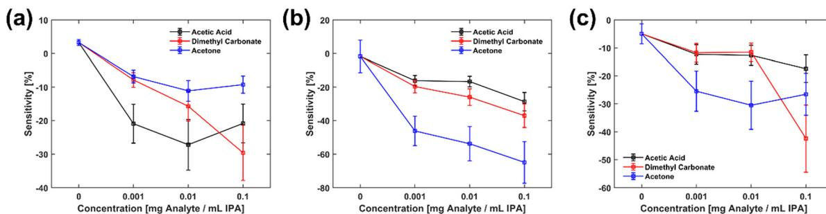
Fig. 5 Responses to analyte in IPA solutions of (a) PDP4T on XLPS/SiO<sub>2</sub> OFETs, (b) **P1BT1:1** on XLPS/SiO<sub>2</sub> OFETs, and (c) P3BT: PDP4T blend (25 : 75 by weight) on XLPS/SiO<sub>2</sub> OFETs. Error bars are standard deviations from three measurements per point.
