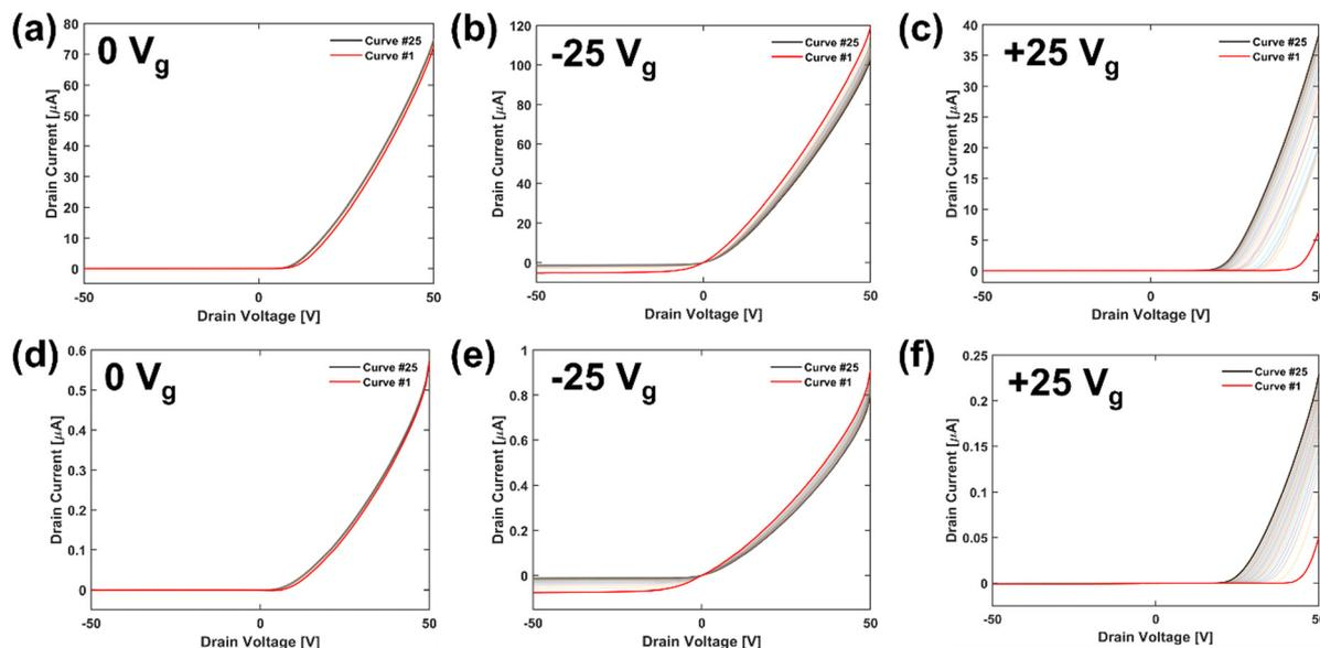
Fig. 6 Two-terminal measurements of PDPP4T on XLPS/SiO<sub>2</sub> OFETs with gate biases of (a) 0 V, (b) –25 V, and (c) +25 V. Two-terminal measurements of P1BT1:1 on XLPS/SiO<sub>2</sub> OFETs with gate biases of (d) 0 V, (e) –25 V, and (f) +25 V.
