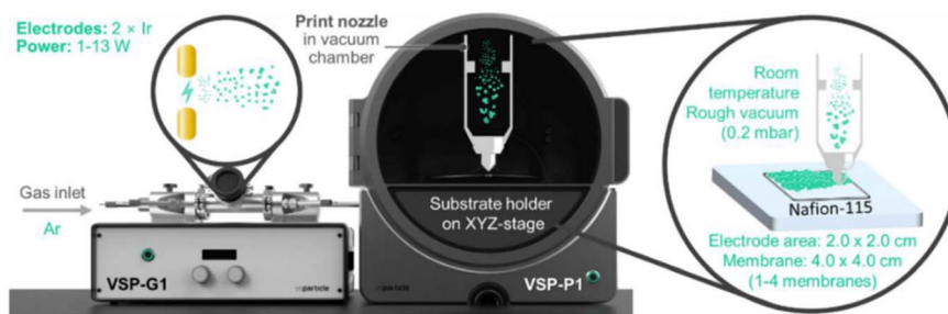
Fig. 5 Schematic of the VSParticle nanoparticle printing technology. A certain wattage is applied to metal electrodes which causes the metal to ablate and particles to detach. The particles agglomerate to form nanoparticles as they are carried by inert Ar to a vacuum chamber where they are printed via a nozzle onto a substrate of choice held by an XYZ-stage. Reproduced with permission from ref. 110. Copyright 2022 MDPI.
