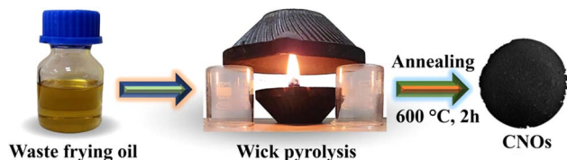
Fig. 6 A schematic illustration for the synthesis of CNOs by the flame pyrolysis method. 77
