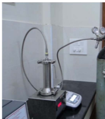
Fig. 2 Nanofiltration experimental set-up.
