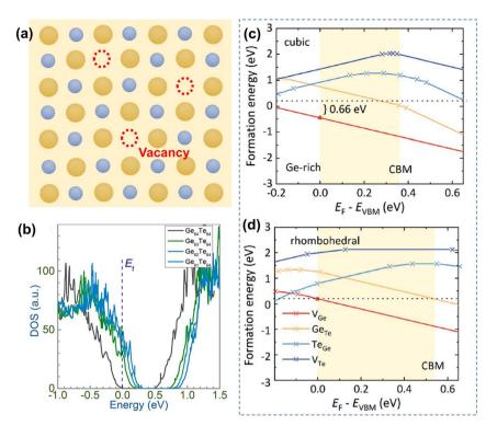
Fig. 8 (a) Schematic view of Ge vacancies in the GeTe matrix. (b) DOS for rhombohedral  $Ge_{64-x}Te_{64}$  with different amounts of Ge deficiencies. The formation energy of atomic defects in (c) cubic and (d) rhombohedral GeTe as a function of the relative Fermi-energy under Ge-rich conditions. (29)
