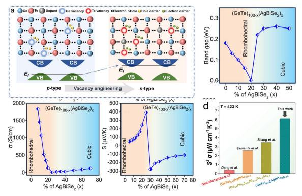
Fig. 13 (a) Schematic diagram of p-type GeTe conversion to n-type.  $^{146}$  Compositional variation of (b) band gap, (c) electrical conductivity, and (d) Seebeck coefficient with the AgBiSe<sub>2</sub> concentration in (GeTe)<sub>100-x</sub>(AgBiSe<sub>2</sub>)<sub>x</sub> (x = 0-50) at room temperature. (e) Comparison of  $S^2\sigma$  of some representative n-type GeTe-based thermoelectric materials.  $^{147}$
