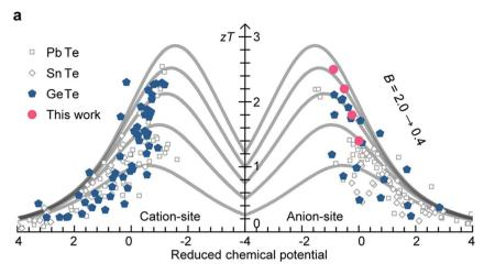
Fig. 25 Comparison of the quality factor (*B*) and figure-of-merit (*ZT*) of GeTe, PbTe, and SnTe thermoelectric materials with cationic and anionic doping.<sup>194</sup>
