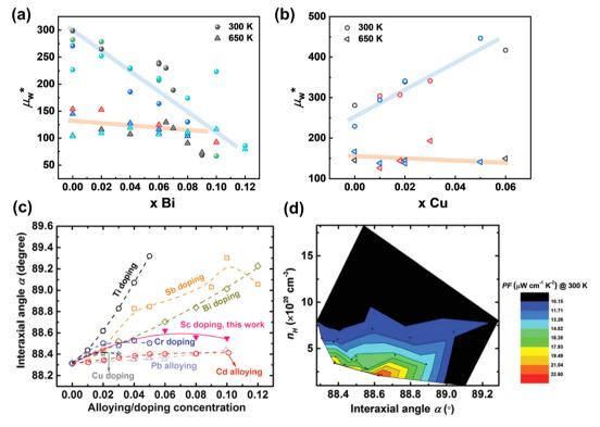
Fig. 12 The weighted mobility for (a) Bi-doped<sup>18,116,141,142</sup> and (b) Cu-doped<sup>51,52,143</sup> GeTe samples. (c) Rhombohedral angle  $\alpha$  as a function of alloying or doping concentration. (d) Contour plot representation of the room-temperature power factor as a function of the rhombohedral angle (interaxial angle)  $\alpha$  and Hall carrier concentration  $n_{\rm H}$ .
