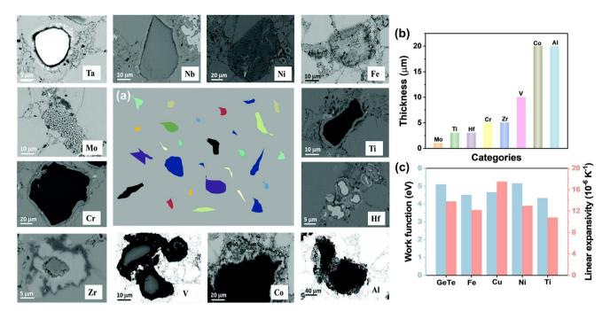
Fig. 22 (a) Microstructures of typical interfaces between GeTe and 12 kinds of pure metals (Cr, Hf, Nb, Ti, Mo, Ni, Ta, Zr, Al, Co, V, and Fe). The central image shows the schematic map of the sample integrating different interfaces. 189 (b) Thickness of reaction layers between GeTe and different pure metals. (c) Work function and linear expansivity of GeTe and some metals as metallization layers.
