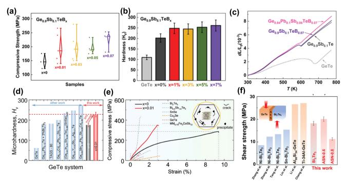
Fig. 24 (a) Compressive strength and (b) Vickers hardness of  $Ge_{0.9}Sb_{0.1}TeB_x$ . (c) Temperature dependence of relative length variation  $(dL/L_0)$ .<sup>33</sup> (d) Comparison of room-temperature Vickers microhardness  $H_v$ . (e) Comparison of compressive tests of GeTe and some other typical brittle thermoelectric materials.<sup>50</sup> (f) Comparison of the shear strength of the segmented legs and some joints.<sup>190</sup>
