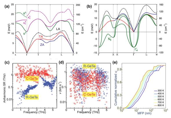
Fig. 4 Phonon-dispersion relations for (a) rhombohedral GeTe and (b) cubic GeTe at 300 K.109 (c) Anharmonic scattering rates (SRs) for rhombohedral and cubic GeTe at 300 K. (d) Group velocity (v) for rhombohedral and cubic GeTe at 300 K.<sup>23</sup> (e) Normalized cumulative lattice thermal conductivity as a function of phonon MFP.30
