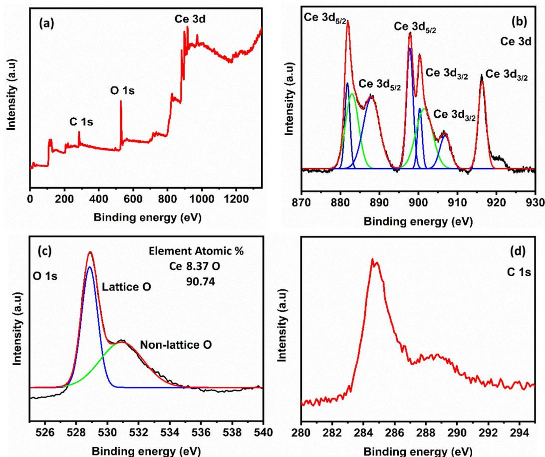
Fig. 4 (a) XPS spectrum of nanocrystalline CeO<sub>2</sub>, (b) high resolution spectrum of Ce 3d, (c) high resolution spectrum of O 1s and (d) high resolution spectrum of C 1s.
