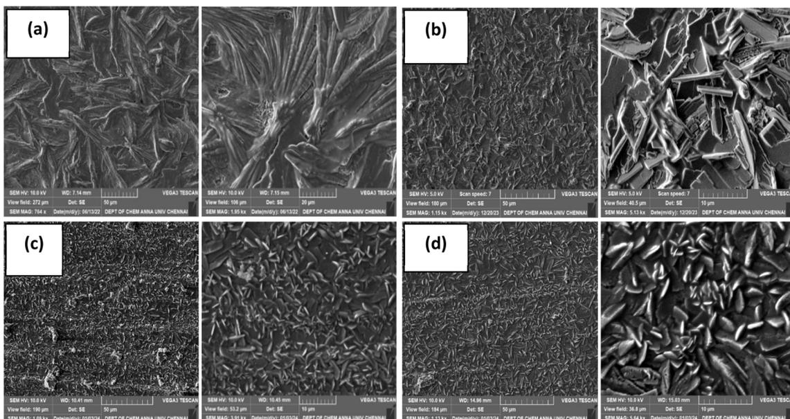
Fig. 7 Surface morphology of zinc phosphate coating formulated with different amounts of nanocrystalline  $\text{CeO}_2$ . (a) ZnP; (b) ZnP-0.3CO; (c) ZnP-0.6CO; and (d) ZnP-0.9CO (right side images are magnified, scale bar = 10  $\mu\text{m}$ ).
