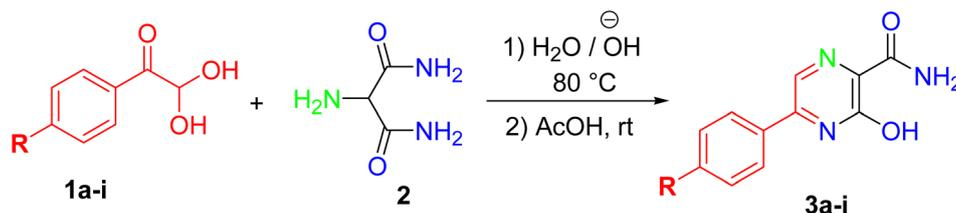
Scheme 7 Synthesis of 3-hydroxy-5-arylpyrazine-2-carboxamide derivatives in aqueous solution.
