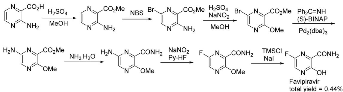
Scheme 2 Favipiravir synthesis according to the strategy developed by Y. Furuta *et al.* (Toyama Chemical Co., Ltd).<sup>28</sup>
