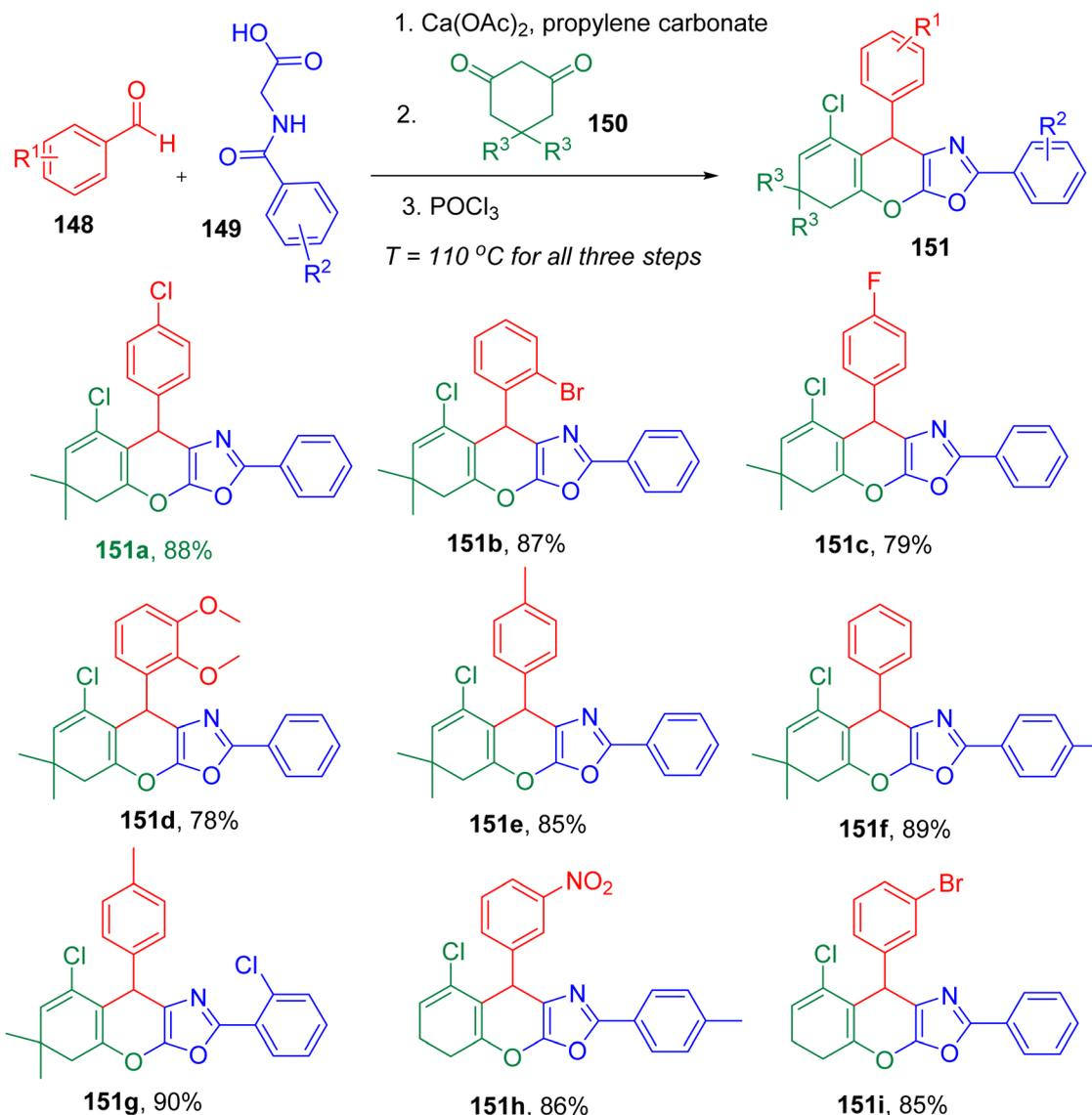
Fig. 38 MCR approach for the synthesis of diverse chromeno[3,2-d]oxazoles derivative.
