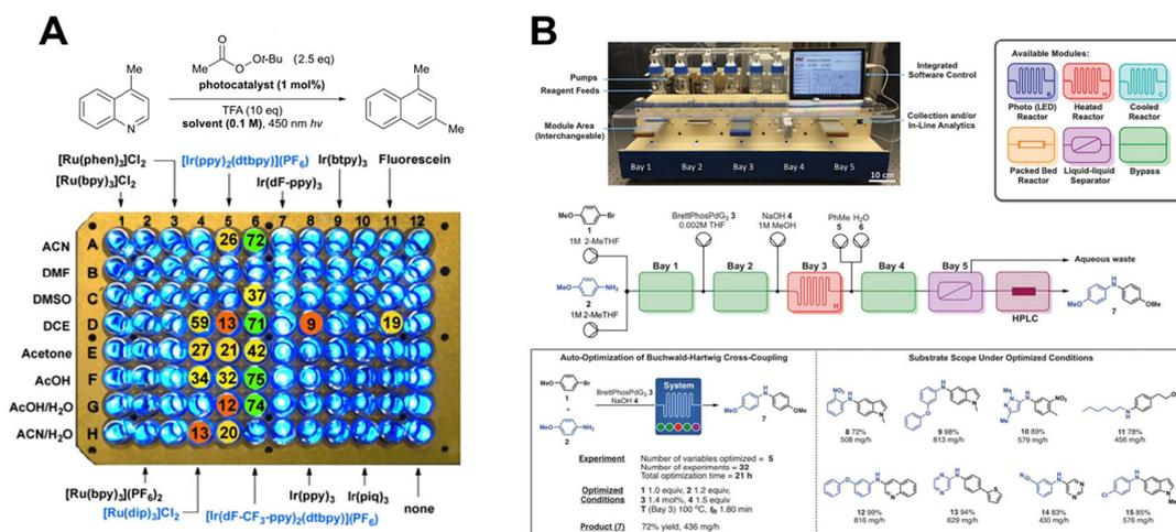
**Fig. 11** Examples of autonomous experimental techniques. (A) HTE applied to photoreaction condition screening. Reprinted with permission request from ref. 111, copyright 2023, Royal Society of Chemistry (B) Flow chemistry systems employed for Buchwald–Hartwig coupling reactions. Reprinted with permission request from ref. 116, copyright 2018, American Association for the Advancement of Science.
