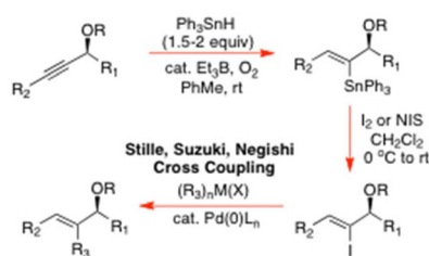
Scheme 1 The rt O -directed free radical hydrostannylative synthesis of ( Z )-trisubstituted alkenes with \text{Ph}_3\text{SnH}/\text{cat. Et}_3\text{B} .
