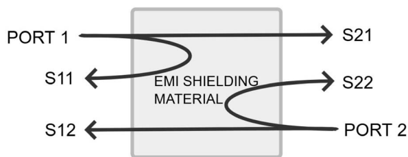
Fig. 2 Complex scattering parameters of an EMIS material from a two-port VNA.
