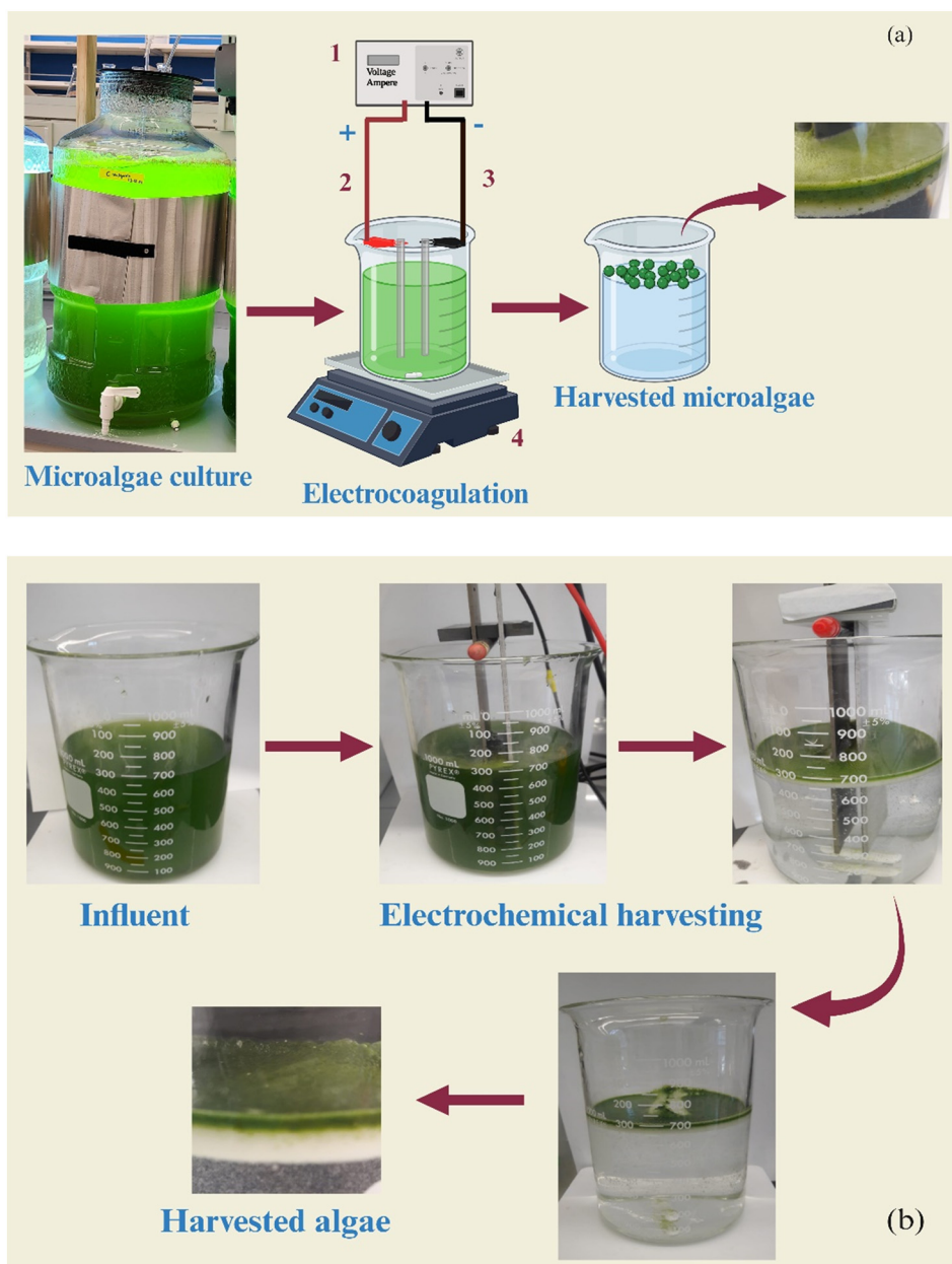
Fig. 1 (a) The schematical diagram of electrocoagulation of algae (1: power supply, 2: anode, 3: cathode, 4: magnetic stirrer); (b) a real application of electrochemical algae harvesting.
