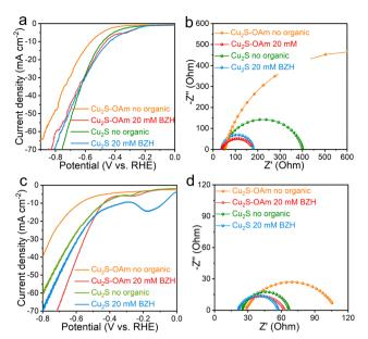
Fig. 3 (a) LSV curves and (b) Nyquist plots at -0.7 V vs. RHE of Cu<sub>2</sub>S-OAm and Cu<sub>2</sub>S in 1 M sodium acetate-acetic acid electrolyte (pH = 5.2) with and without BZH at room temperature; (c) LSV curves and (d) Nyquist plot at -0.7 V vs. RHE of Cu<sub>2</sub>S-OAm and Cu<sub>2</sub>S in 1 M potassium carbonatepotassium bicarbonate electrolyte (pH = 9) with or without BZH at room temperature
