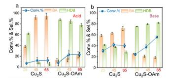
Fig. 5 BZH conversion and selectivity toward BA and HDB after 20 min reaction on  $Cu_2S$  and  $Cu_2S$ –OAm electrodes at -0.8 vs. RHE, 25 °C, 45 °C or 65 °C in (a) 1 M sodium acetate–acetic acid solution (pH = 5.2) with 20 mM BZH; (b) 1 M potassium carbonate–potassium bicarbonate solution (pH = 9.0) with 20 mM BZH.
