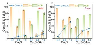
Fig. 4 BZH conversion and selectivity toward BA and HDB after 20 min reaction on  $Cu_2S$  and  $Cu_2S$ -OAm electrodes at 0.4, -0.8, -1.0 V vs. RHE, 25 °C in (a) 1 M sodium acetate-acetic acid solution (pH = 5.2) with 20 mM BZH; (b) 1 M potassium carbonate-potassium bicarbonate solution (pH = 9.0) with 20 mM BZH.
