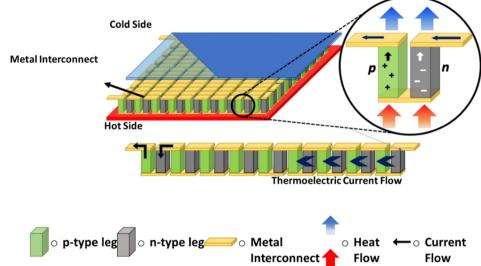
Fig. 4 Diagram depicting the internal structure of various p-type and n-type legs in thermoelectric power generators.
