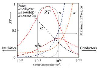
Fig. 5 Thermoelectric parameters with variations in carrier concentration taken from ref. 50, where  $\alpha$  represents the Seebeck coefficient,  $\sigma$  represents the electrical conductivity, k represents the thermal conductivity, and ZT represents the figure of merit. The image was adapted with permission from Prasad et al., 51 Springer Nature 2020.
