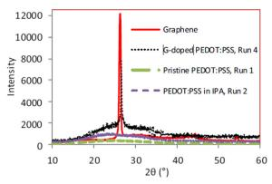
Fig. 10 XRD patterns of graphene, pristine PEDOT:PSS thin film (run 1), PEDOT:PSS thin film prepared using IPA as a co-solvent (run 2), and SVACfabricated graphene-doped PEDOT:PSS (run 4).180
