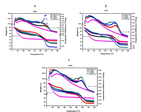
Fig. 6 TGA-DTA profile of (a) MTH, (b) ETH and (c) PTH conversion at  $T=350~{\rm ^{\circ}C}$  and WHSV = 7 h $^{-1}$ .
