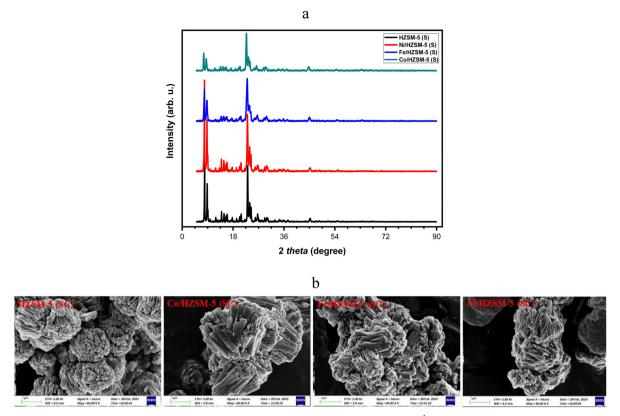
Fig. 7 (a) XRD pattern and (b) SEM images of spent catalysts (operating condition: 350  $^{\circ}$ C and 7 h<sup>-1</sup>).
