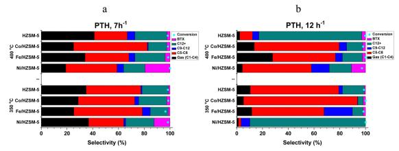
Fig. 3 (a) and (b) Product distribution and propanol conversion in the PTH process.
