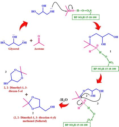
Scheme 1 Proposed mechanism of glycerol acetalization using the BP-SO<sub>3</sub>H-15-18-100 catalyst.
