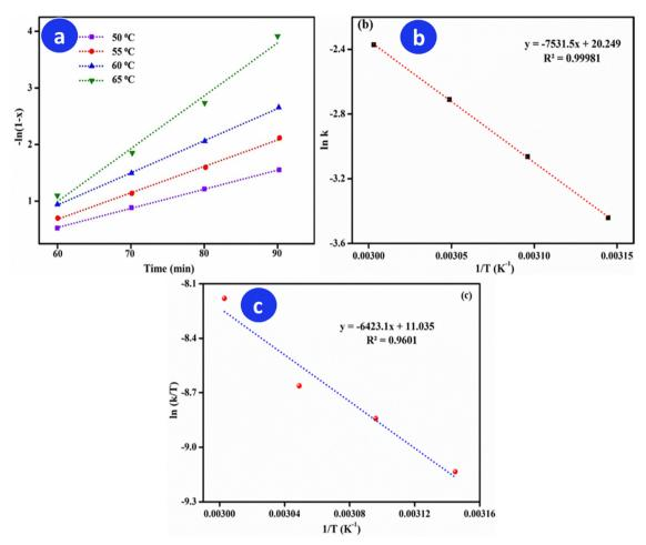
Fig. 4 (a) Plot of  $-\ln(1-X)$  vs. time, where X = glycerol conversion at different temperatures for acetalization reaction, (b) the corresponding Arrhenius plot of  $\ln k$  vs. 1/T, and (c) thermodynamic behaviour of acetalization reaction.
