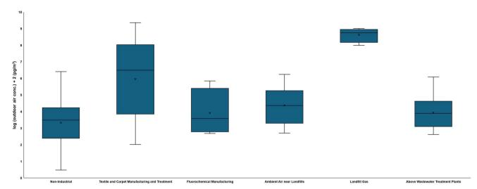
Fig. 4 Box and whisker plot comparison between min and max of reported FTOH outdoor air concentration at different sites. The non-industrial data are obtained from ref. 70
