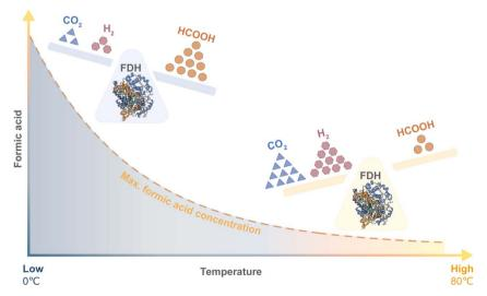
Fig. 4 Concentrations of dissolved formic acid in equilibrium with  $CO_2$  and hydrogen at different temperatures. At lower temperatures, the equilibrium favours formic acid formation, which in turn, creates a more acidic environment. But would require a catalyst that is able to operate at low temperatures, such as enzymes (FDH).
