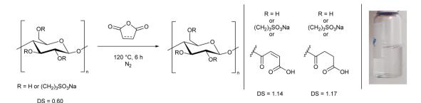
Scheme 2 Synthesis of water-soluble cellulose derivatives from the reaction of sulfonated cellulose (Scheme 1) with either maleic or succinic anhydride. The DS and an example solution are shown.
