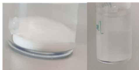
Fig. 3 The interaction of sulfonated cellulose with water. Left: water-repellent behaviour, and right: the formed suspension.
