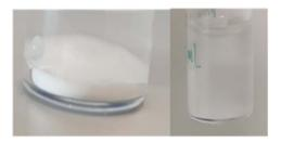
Fig. 3 The interaction of sulfonated cellulose with water. Left: waterrepellent behaviour, and right: the formed suspension.
