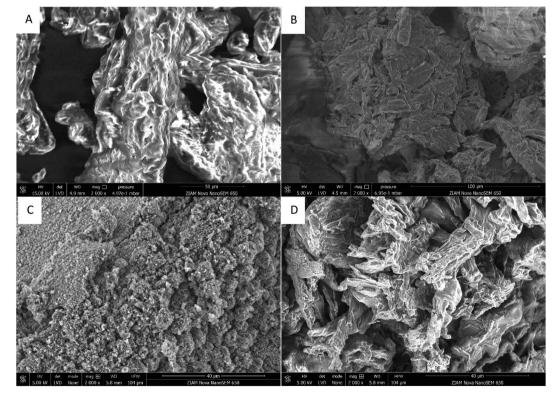
Fig. 4 SEM images at  $2000 \times$  magnification of microcrystalline cellulose (A), 1,3-propane sultone modified cellulose (B), water-soluble cellulose with maleic anhydride substituents (C), and water-soluble cellulose with succinic anhydride substituents (D).
