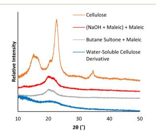
Fig. 5 XRD patterns of cellulose, and differently modified cellulose analogues (from Schemes 2 and 3).
