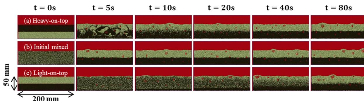
Fig. 12 Time series of images of CFD-DEM simulations with only gas flow for different initial particle configurations (a)–(c).
