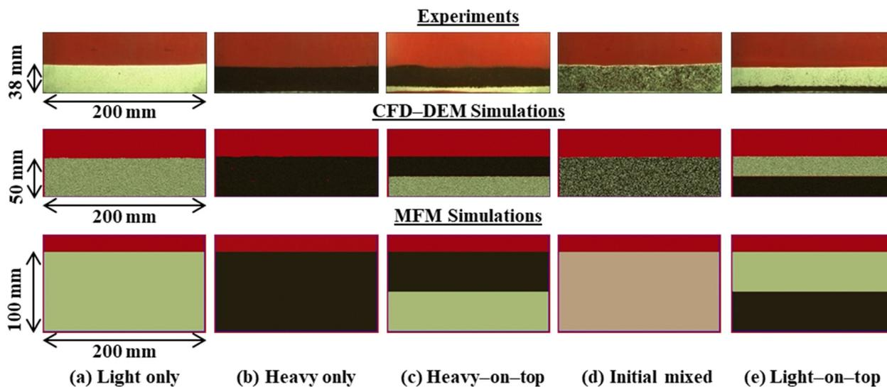
Fig. 2 Optical images of different initial conditions (a)–(e) that are used in experiments, CFD-DEM simulations and MFM simulations. In experiments, the initial fill height of particles is 50 mm, but the bottom 12 mm of particles of the bed cannot be observed due to a horizontal plate that joins the fluidized bed to the gas distributor.
