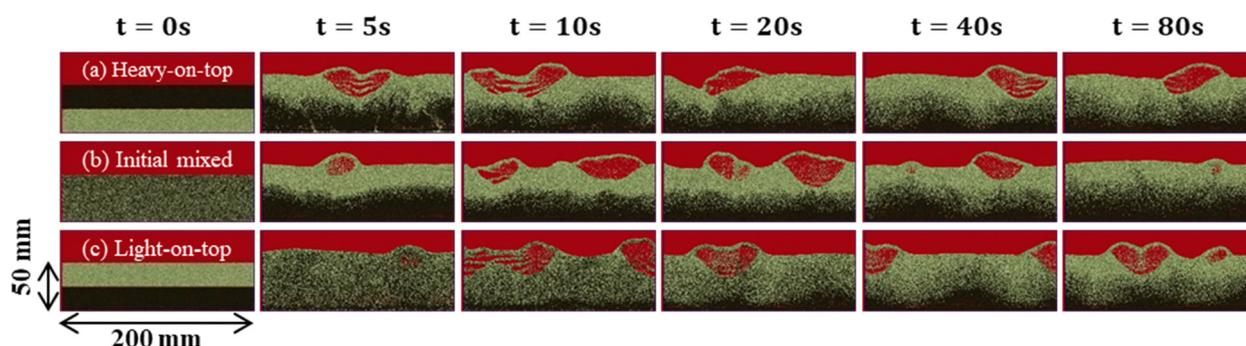
Fig. 10 Time series of images of CFD-DEM simulations with combined gas flow and vibration for different initial particle configurations (a)–(c).
