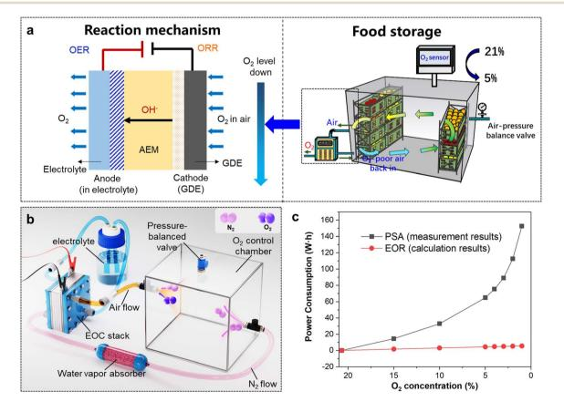
Fig. 3 (a) Illustrations of the working mechanism of the EOR when applied in food storage. (b) Simulation diagram showing the structural configuration of the designed EOR system. (c) Energy consumption of different  $O_2$  removal devices: the results for PSA were obtained through practical measurements, while the results for EOR were calculated under simulation conditions.
