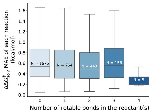
Fig. 8 Distribution of the  $\Delta\Delta G_{\text{sol}}^{\ddagger}$  MAE categorized by the number of rotatable bonds found in the reactant(s) of each reaction (outliers not shown). The  $N$  indicates the number of reactions in each distribution. The fine-tuned model without additional feature tested on the pre-training set reaction split.
