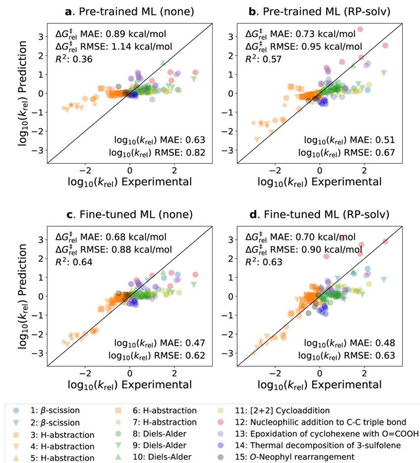
Fig. 5 Parity plots of the predicted vs. experimental  $k_{\text{rel}}$  values. (a) The pre-trained model with no additional  $k_{\text{rel}}$  feature. (b) The pre-trained model with the RP-solv feature. (c) The fine-tuned model with no additional feature. (d) The fine-tuned model with the RP-solv feature. The errors are reported in both  $\log_{10}(k_{\text{rel}})$  and  $\Delta G_{\text{rel}}^{\ddagger}$  units, and  $R^2$  represents the coefficient of determination.
