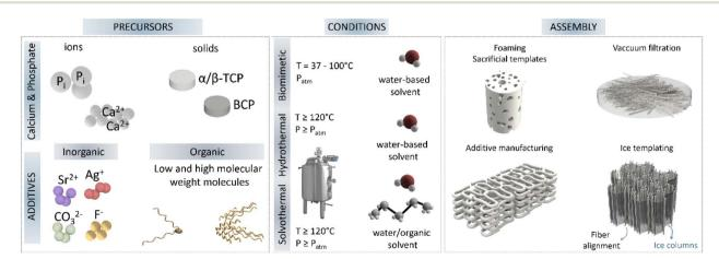
Fig. 6 Main synthesis routes for nanostructure HA, highlighting the precursor sources often used, together with common additives, the conditions frequently used to synthesise high aspect ratio HA; and finally, the common 3D assembly strategies to obtain 3D ceramics (TCPtricalcium phosphate, BCP-biphasic calcium phosphate).
