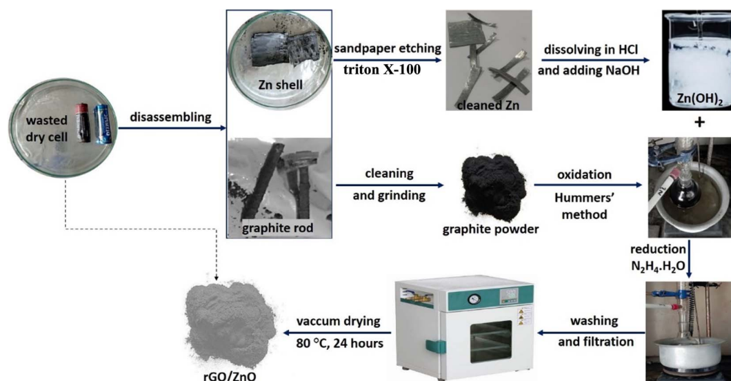
Scheme 1 Synthesis of rGO/ZnO utilizing graphite and Zn collected from wasted dry cells.
