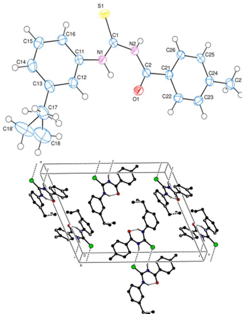
Fig. 4 Molecular structure of compound ES-2 where thermal ellipsoid is drawn at the 50% probability level b: a partial packing diagram viewed along the *c*-axis. Hydrogen bonds are shown as dashed lines. Sulfur green, oxygen red, nitrogen blue.
