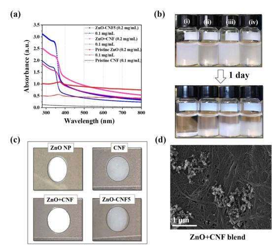
Fig. 18 (a) UV-visible absorption spectroscopic analysis of ZnO–CNF5 hybrid, ZnO + CNF blend, and ZnO NP at 0.1 mg mL $^{-1}$  and 0.2 mg mL $^{-1}$  and pristine CNF sample at 0.1 mg mL $^{-1}$ , (b) dispersion stability at a high concentration such as (0.5 mg mL $^{-1}$ ) (i) ZnO NP, (ii) pristine CNF, (iii) ZnO + CNF blend and (iv) ZnO–CNF5 hybrid, (c) the whitening effect drop-casted on the glass slide, (d) FE-SEM images of ZnO + CNF blend after dry. $^{165}$
