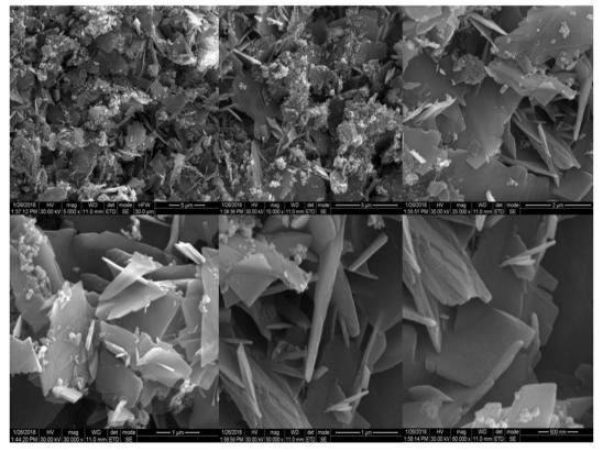
Fig. 2 FE-SEM morphology of ZnO nanoflakes.<sup>30</sup>
