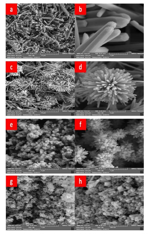
Fig. 7 Typical FE-SEM prepared ZnO samples (a) and (b) hexagonal rods (ZnO-1), (c) and (d) flower-like rods (ZnO-2), (e) and (f) flowers-like prismatic (ZnO-3), (g) and (h) quasi-prismatic (ZnO-4).<sup>51</sup>
