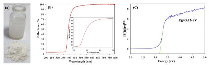
Fig. 20 Optical properties of ZnO NPs: (a) white color of ZnO NPs, (b) UV-visible diffuse reflectance spectra of ZnO NPs (inset: zoomed in spectra in the range from 350 to 500 nm), and (c) plot of  $[F(R)h_{-}]0.5$  against photon energy (hv).<sup>168</sup>
