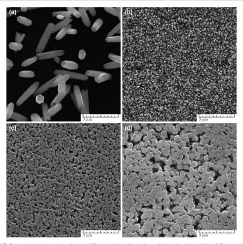
Fig. 5 SEM images of ZnO nanostructures synthesized at different origin of seed layer: (a) on clear glass, (b) on MS seeds, (c) on ED seeds, (d) on AD seeds. Other parameters were: 0.1 M Zn(NO<sub>3</sub>)<sup>2+</sup> HMTA equimolar solution, t = 3 h, T = 90 °C.<sup>50</sup>
