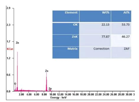
Fig. 3 EDX spectrum of ZnO nanoflakes.30
