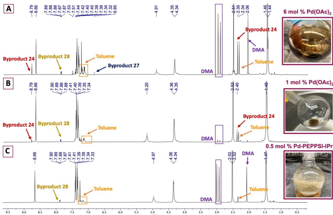
Fig. 2 <sup>1</sup>H NMR and photographic comparison of crude **10** formed using: (A) 6 mol% Pd(OAc)<sub>2</sub>; (B) 1 mol% Pd(OAc)<sub>2</sub>; (C) 0.5 mol% Pd-PEPPSI-IPr. Residual reaction solvent, DMA, and azeotroping solvent, toluene, are indicated.
