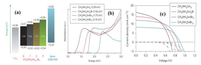
Fig. 14 (a) Band-gap modulation; (b) absorbance; and (c) performance with respect to the variation of bromine in the X-site of MASn( $I_{1-x}$ -Br<sub>x</sub>)<sub>3</sub> perovskite. Reproduced from ref. 123 with permission from Springer Nature. Copyright 2014.
