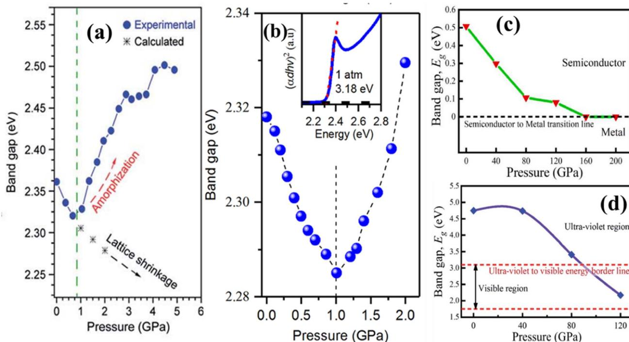
Fig. 15 Pressure-induced band-gaps for MAPbBr<sub>3</sub>, CsPbBr<sub>3</sub>, CsYbCl<sub>3</sub> and KCaCl<sub>3</sub>.<sup>135–138</sup> (a) Reproduced from ref. 135 with permission from ACS, copyright 2015. (b) Reproduced from ref. 136 with permission from ACS, copyright 2017. (c) Reproduced from ref. 137 with permission from Elsevier, copyright 2022. (d) Reproduced from ref. 138 with permission from RSC, copyright 2021.
