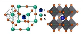
Fig. 6 The basic structure of ABX<sub>3</sub> with corner-sharing BX<sub>6</sub> octahedral.
