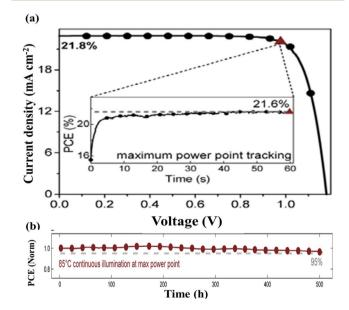
Fig. 9 (a) Photovoltaic performance of the PSC with a configuration of FTO/c&m-TiO<sub>2</sub>/perovskite/spiro-OMeTAD/Au and (b) stability. Reproduced from ref. 101 with permission from *Science*, copyright 2016.
