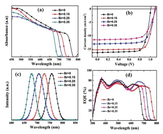
Fig. 13 (a) Absorbance; (b) current density; (c) intensity and (d) quantum efficiency of the device with ITO/PEDOT:PSS/MA $_{0.85}$ Cs $_{0.15}$ Pb( $I_{1-x}$ Br $_x$ ) $_3$ / PC $_{61}$ BM/BCP/Ag, measured under 1 sun conditions (100 mW cm $^{-2}$ , AM 1.5G). Reproduced from ref. 122 with permission from WILEY-VCH Verlag GmbH & Co. KGaA, Weinheim, copyright 2019.
