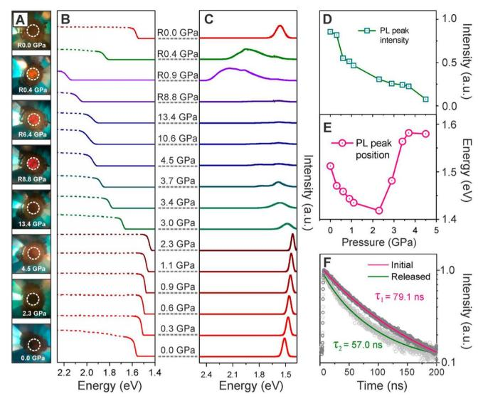
Fig. 16 (A) Snapshots of FAPbl<sub>3</sub> NCs in a DAC at various pressures. (B) Absorption and (C) PL spectra under pressure. (D) PL peak intensity evolution before complete amorphization. (E) PL peak position evolution before complete amorphization. (F) PL lifetime decay curves of the FAPbl<sub>3</sub> NCs before and after pressure. Reproduced from ref. 144 with permission from ACS, copyright 2018.
