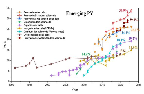
Fig. 1 The recent progress of emerging photovoltaic solar cells. Data extracted from NREL (https://www.nrel.gov/).
