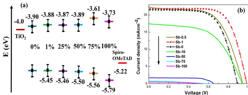
Fig. 12 (a) Band-gap modulation; (b) the influence of band-gap modulation on the photovoltaic performance metrics of the PSCs with  $\text{MAPb}_{1-x}\text{Sb}_{2x/3}\text{I}_3$ . Reproduced from ref. 116 with permission from ACS, copyright 2016.
