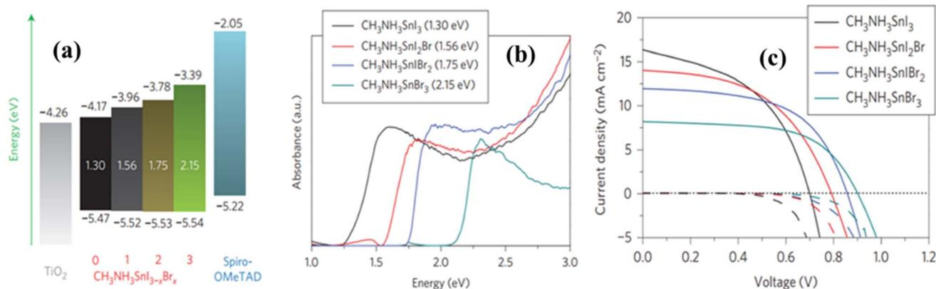
Fig. 14 (a) Band-gap modulation; (b) absorbance; and (c) performance with respect to the variation of bromine in the X-site of MASn(I<sub>1-x</sub>Br<sub>x</sub>)<sub>3</sub> perovskite. Reproduced from ref. 123 with permission from Springer Nature. Copyright 2014.
