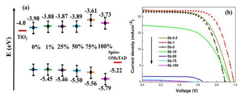
Fig. 12 (a) Band-gap modulation; (b) the influence of band-gap modulation on the photovoltaic performance metrics of the PSCs with MAPb<sub>1-x</sub>Sb<sub>2x/3</sub>l<sub>3</sub>. Reproduced from ref. 116 with permission from ACS, copyright 2016.
