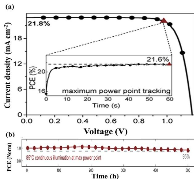
Fig. 9 (a) Photovoltaic performance of the PSC with a configuration of FTO/c-TiO<sub>2</sub>/perovskite/spiro-OMeTAD/Au and (b) stability. Reproduced from ref. 101 with permission from *Science*, copyright 2016.
