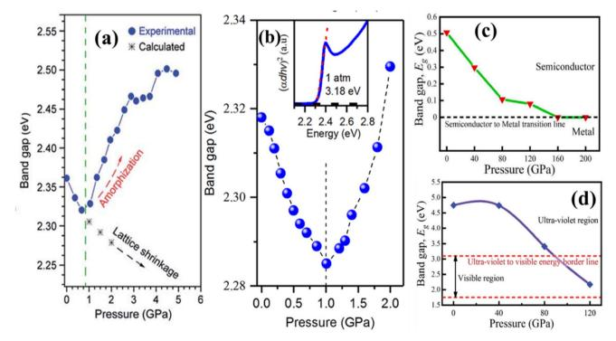
Fig. 15 Pressure-induced band-gaps for MAPbBr<sub>3</sub>,  $CsPbBr_3$ ,  $CsPbBr_3$ ,  $CsPbBr_3$ ,  $CsPbBr_3$  and  $KCaCl_3$ . Index Scale Scale
