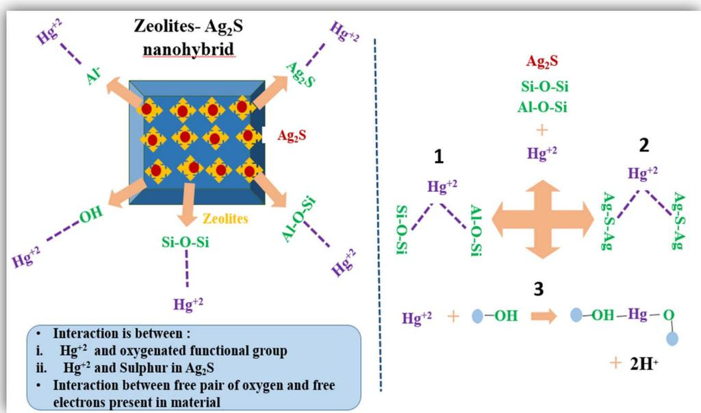
Fig. 8 Major processes of mercury adsorption in zeolite-Ag<sub>2</sub>S nanohybrid materials from wastewater. The proposed chemical reaction mechanism: (1) and (2) represent physisorption and (3) represents chemisorption. Reproduced with permission from ref. 178. Copyright [2023], Elsevier. All rights are reserved.
