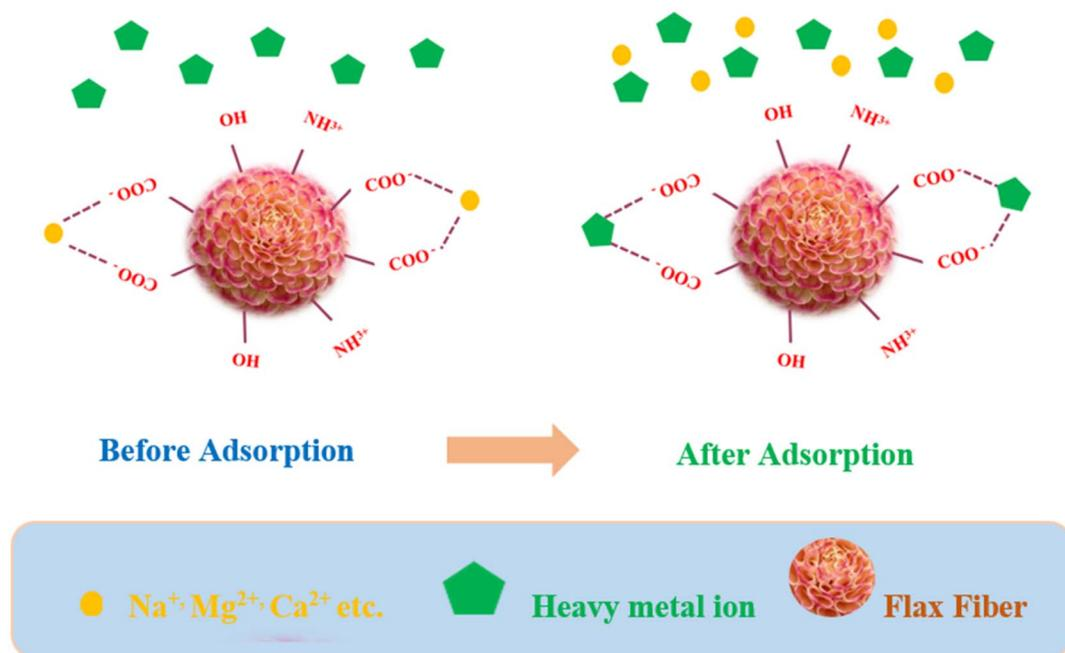
Fig. 7 Schematic illustration of proposed mechanisms for heavy metal adsorption on flax fiber towels.<sup>109</sup>
