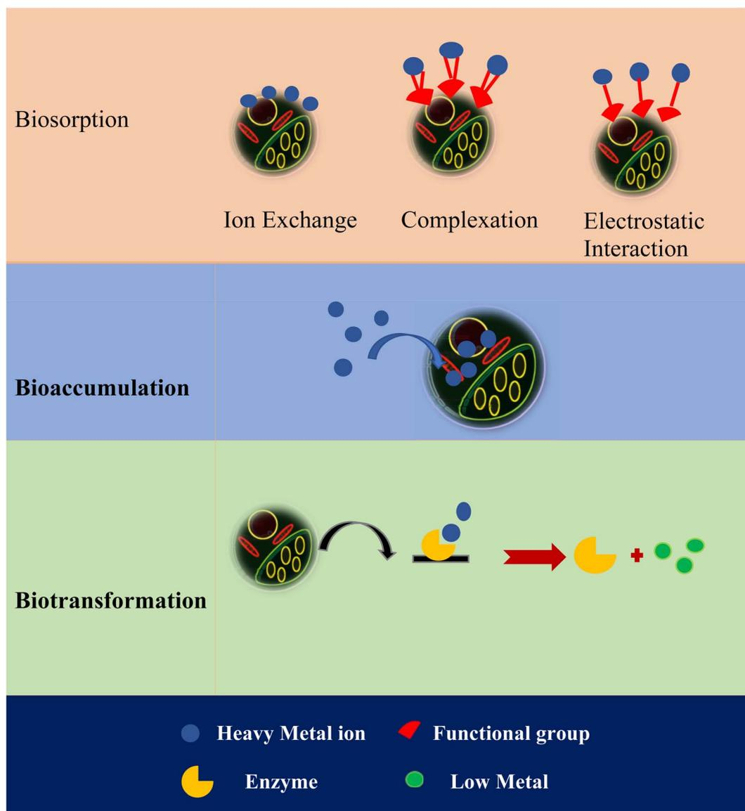
Scheme 1 Mechanism for the removal of heavy metals by algae.<sup>34</sup>
