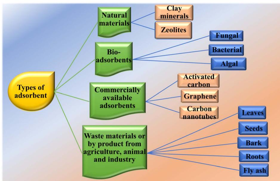
Fig. 4 Types of adsorbent and their sources.
