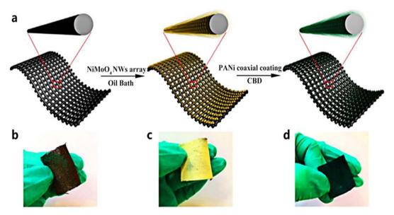
Fig. 13 (a) Representation of a fabrication process for carbon cloth/PANI/NiMoO<sub>4</sub>, (b) digital photo of pristine carbon cloth, and (c) digital view of carbon cloth/PANI/NiMoO<sub>4</sub> and (d) final product of carbon cloth/PANI/NiMoO<sub>4</sub> [Reproduced with permission from ref. 242. A copyright of Elsevier, 2015].
