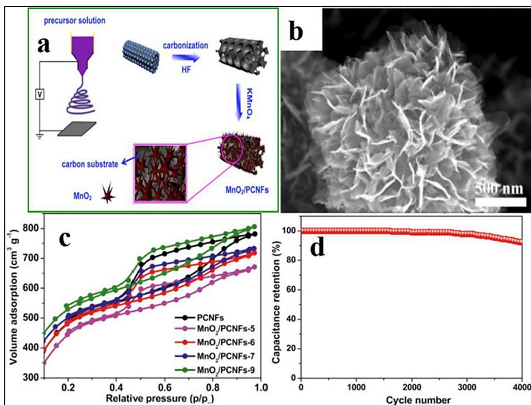
**Fig. 9** (A) Design for the preparation of the MnO<sub>2</sub>/PCNF composite, (b) SEM of the MnO<sub>2</sub>/PCNF composite, (c) isotherm for nitrogen adsorption and desorption of PCNFs and MnO<sub>2</sub>/PCNF composite, and (d) cycling stability of MnO<sub>2</sub>/PCNFs as an electrode over  $4.0 \times 10^3$  cycles at a current of 0.5 A g<sup>-1</sup> [Reproduced with permission from ref. 55. A copyright of Elsevier, 2019].
