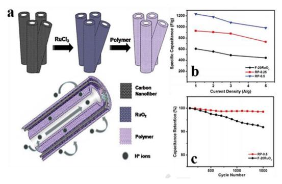
Fig. 8 (a) Steps for the production of double-walled CNFs modified with ruthenium dioxide and poly(benzimidazole). (b) Specific capacitance of F-20 RuO<sub>2</sub>, RP-0.25, and RP-0.5 at different current densities from 1.0 to 5.0 A  $g^{-1}$ , and (c) electrochemical action of the materials RP-(0.5) and F-(20) RuO<sub>2</sub> in terms of stability for 1500 cycles when the amount of current is 1.0 A  $g^{-1}$ . [Reproduced with permission from ref. 125. A copyright of RSC, 2013].
