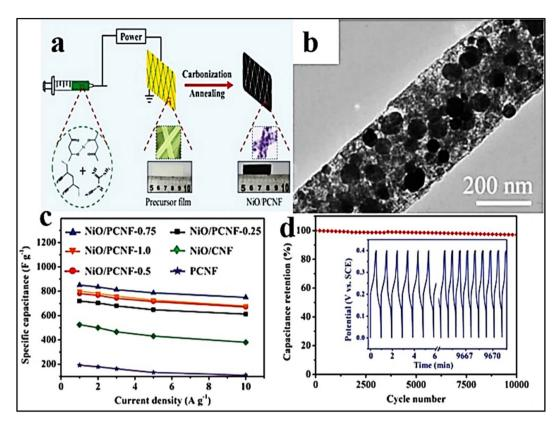
Fig. 10 (a) Fabrication process of the composite made of NiO and PCNF, (b) TEM surface morphology of NiO/PCNF-(0.75), (c) electrical capacity of NiO/PCNF at a composition of 0.25, 0.5, 0.75, and 1.0 against current density (A  $g^{-1}$ ), and (d) NiO/PCNF-(0.75) cycling stability at a 10 A  $g^{-1}$  for 10 000 cycles [Reproduced with permission from ref. 157. A copyright of Wiley, 2018].
