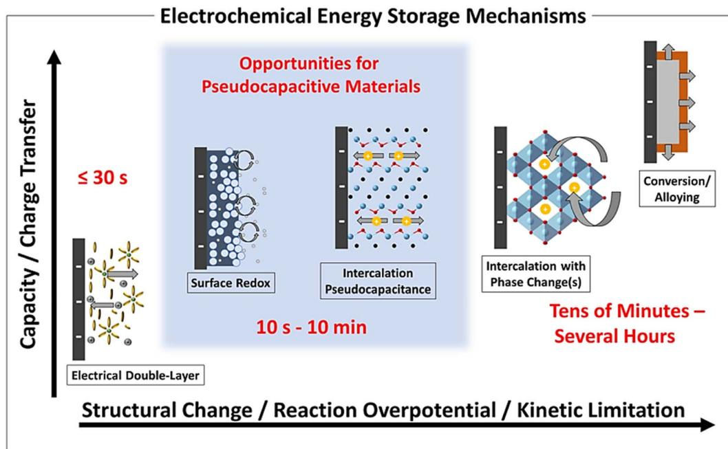
Fig. 3 Different electrochemical energy harnessing mechanisms of PCs as a function of characteristic capacity, degree of structural modifications in the electrodes, reaction over-potential, and limits of the chemical kinetics [Reproduced with permission from ref. 30. A copyright of ACS, 2020].
