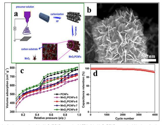
Fig. 9 (A) Design for the preparation of the  $MnO_2/PCNF$  composite, (b) SEM of the  $MnO_2/PCNF$  composite, (c) isotherm for nitrogen adsorption and desorption of PCNFs and  $MnO_2/PCNF$  composite, and (d) cycling stability of  $MnO_2/PCNF$ s as an electrode over  $4.0 \times 10^3$  cycles at a current of 0.5 A  $g^{-1}$  [Reproduced with permission from ref. 55. A copyright of Elsevier, 2019].
