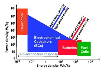
Fig. 1 Ragone graph of power density vs. energy density (ED) for different ESDs [Reproduced with permission from ref. 2. A copyright of
