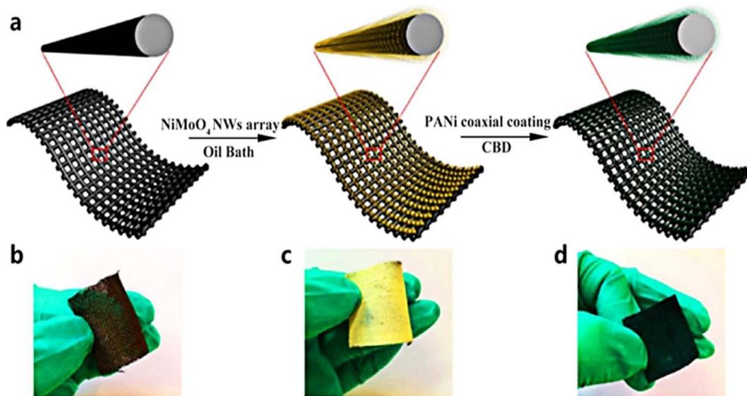
Fig. 13 (a) Representation of a fabrication process for carbon cloth/PANI/NiMoO<sub>4</sub>, (b) digital photo of pristine carbon cloth, and (c) digital view of carbon cloth/PANI/NiMoO<sub>4</sub> and (d) final product of carbon cloth/PANI/NiMoO<sub>4</sub> [Reproduced with permission from ref. 242. A copyright of Elsevier, 2015].
