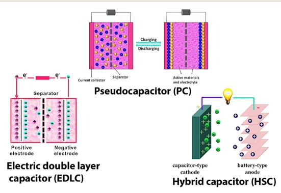
Fig. 2 Working and internal structure of different types of SCs.
