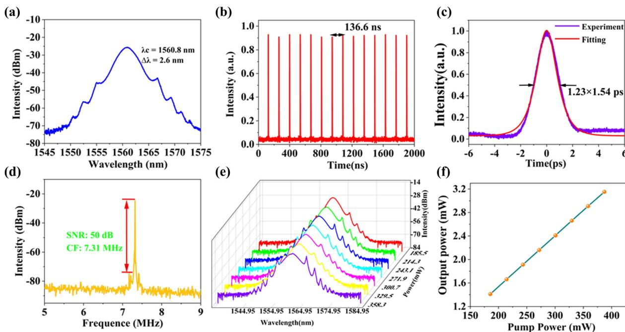
Fig. 6 (a) Optical spectrum of conventional soliton mode-locking; (b) oscilloscope tracking of the mode-locking pulse train; (c) autocorrelation trace with a  $\text{sech}^2$  fitting; (d) the RF spectrum of mode-locking pulses; (e) spectral evolution at different pump powers; (f) output power at different pump power.
