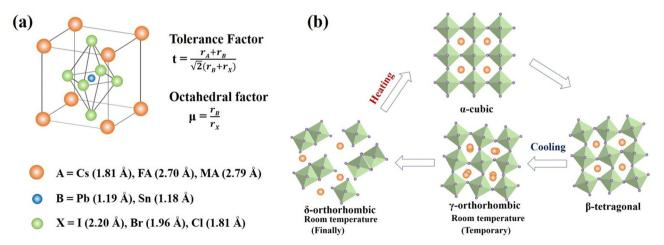
Fig. 1 (a) A cubic perovskite crystal structure (α-phase) showing flexibility in the choice of cation (A), metal (B), and anion (X), whose ionic radii are shown. (b) Schematic presentation of the structural phase transition of various polymorphs of CsPbl3 as a function of temperature.
