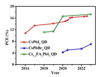
Fig. 21 The PCE evolution of PQD solar cells.
