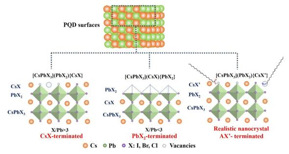
Fig. 4 Idealized surface termination models for the as-synthesized CsPbX<sub>3</sub> QDs
