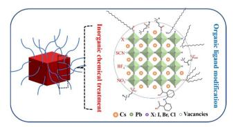
Schematic illustration of the ligand-capped PQDs and an enlarged view of the nanocrystal surface with defects and different types of surface ligands used for the stabilization of PQDs
