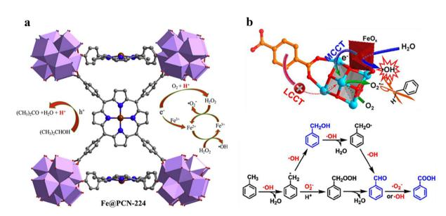
Fig. 17 (a) Proposed mechanism of oxygen-related radical generation in photocatalytic systems with Fe@PCN-224. Adapted with permission from ref. 195. Copyright 2018, Elsevier. (b) Schematic illustration showing the conversion of  $H_2O$  to 'OH by visible light-driven MCCT process over Fedoped UiO-66 and proposed catalytic mechanism of toluene oxidation. Adapted with permission from ref. 87. Copyright 2019, the American Chemical Society.
