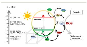
**Fig. 14** General illustration of possible reactive oxygen species (ROS) in MOF-based photocatalysts responsible for oxidation reactions under an aqueous and aerobic conditions.<sup>171</sup>
