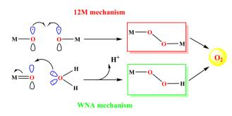
**Fig. 11** Schematic representation of the two mechanistic pathways for O–O bond formation for single-site (solvent water nucleophilic attack, WNA) and dinuclear (interaction of two M–O units, I2M) artificial oxygen evolutions catalysts (OECs).
