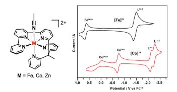
**Fig. 11** Cyclic voltammograms of Fe<sup>II</sup> and Co<sup>II</sup> polypyridyl complexes. Reproduced with permission from ref. 64. Copyright 2022 American Chemical Society.
