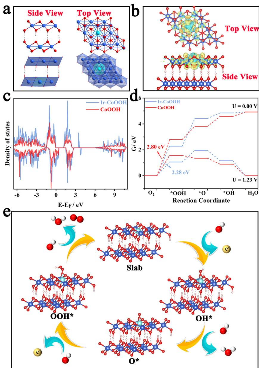
**Fig. 6** (a) Top and side view crystal structures of Ir-CoOOH, (b) charge density difference over Ir-CoOOH, (c) DOS of Ir-CoOOH and CoOOH (Fermi level is set as 0 eV), (d) Gibbs free energy diagrams of the 4-electron OER process for the Ir-CoOOH and CoOOH catalysts at an applied overpotential of 1.23/0.00 V vs. RHE, (e) the proposed 4-electron OER mechanism for the Ir-CoOOH catalyst.
