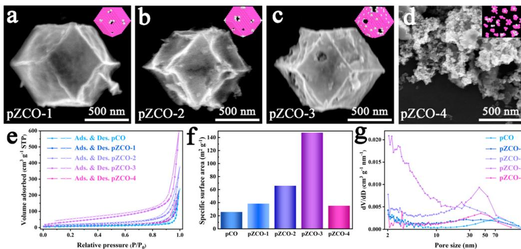
Fig. 1 (a–d) SEM images of the pZCO series. (e–g) N<sub>2</sub> sorption isotherms, BET specific surface area analysis and the corresponding PSD curves of the pCO and pZCO series.
