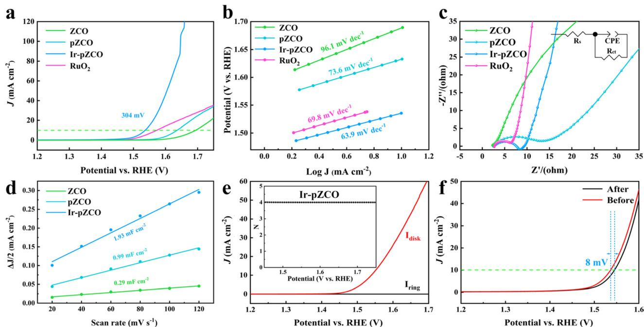
**Fig. 4** (a) LSV curves, (b) Tafel plots, (c) EIS analysis, and (d)  $C_{dl}$  values of all samples. (e) RRDE voltammogram and the calculated  $N$  for Ir-pZCO. (f) LSV curves of Ir-pZCO before and after a 10-hour OER.
