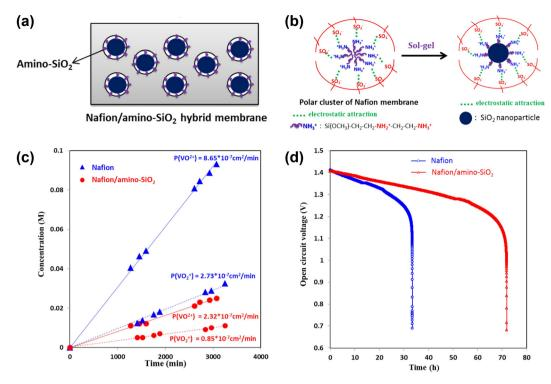
Fig. 6 (a) Schematic illustration of Nafion/inorganic hybrid membrane. (b) Preparation of Nafion/amino-SiO<sub>2</sub> hybrid membrane. (c) Effect of Nafion and Nafion/amino-SiO<sub>2</sub> membrane on intracellular VO<sup>2+</sup> and VO<sub>2</sub>+ concentration. (d) OCV of VRFB over time using Nafion and Nafion/amino-SiO<sub>2</sub> membrane in the charged state of 75%. Reproduced from ref. 92 with permission from Elsevier, Copyright 2015.
