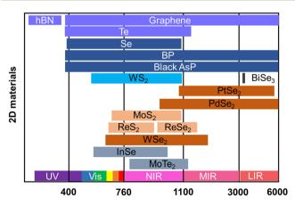
Fig. 3 Relationship between 2D materials and the corresponding detection bands. Reproduced with permission from ref. 69. Copyright 2021, Wiley-VCH.
